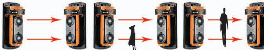
One or Two Beams Are Interrupted
